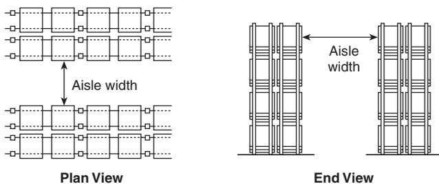
**FIGURE A.3.3.7 Illustration of Aisle Width.** [13:Figure A.3.9.3.1]
