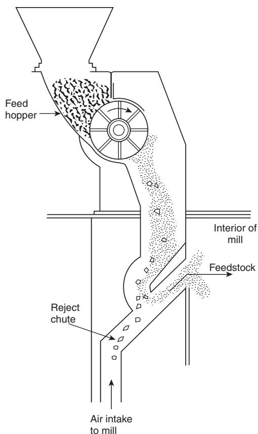
**FIGURE A.40.4.1.2.3(a) Pneumatic Separator. [654: Figure A.9.1.2.3(a)]**
