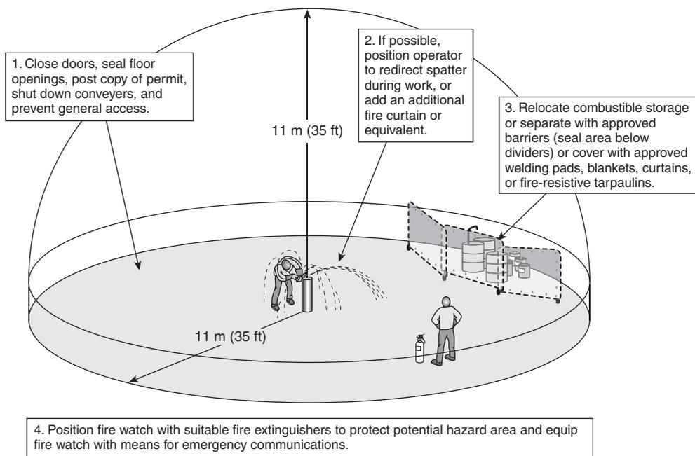
FIGURE A.41.3.5.1(1)(a) The 35 Foot Rule Illustrated. [51B:Figure A.5.5.1(1)(a)]
