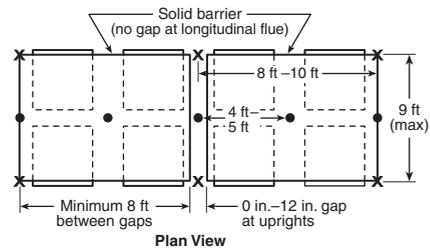
**FIGURE 66.16.6.1.1(b) Double-Row Rack Sprinkler Layout for Design Scheme “A.” [30: Figure 16.6.1.1(b)]**
