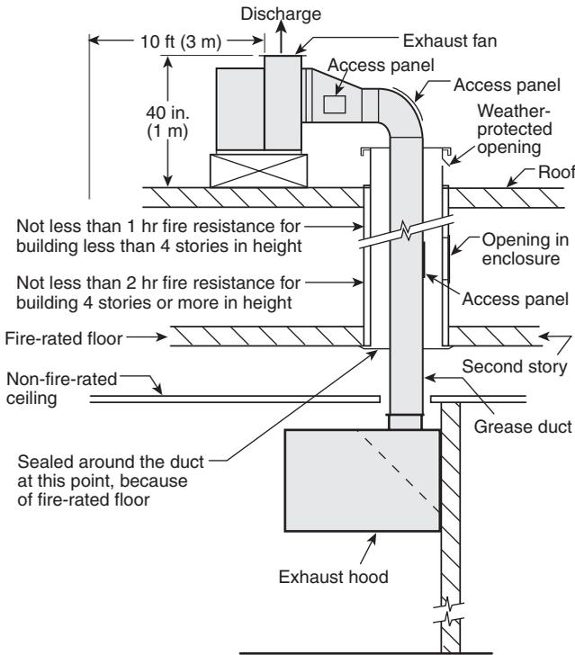
**FIGURE A.50.2.2(c) Typical Section View for Building with Two Stories or More with Non-Fire-Rated Ceiling and Fire-Rated Floor. [Clearances given in Figure A.50.2.2(a) apply also to this drawing.] [96:Figure A.4.2(c)]**
