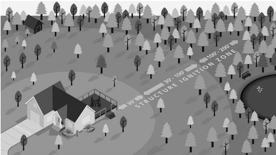
**FIGURE A.17.1.8 The Structure Ignition Zone. [1144:Figure A.4.2.4]**
